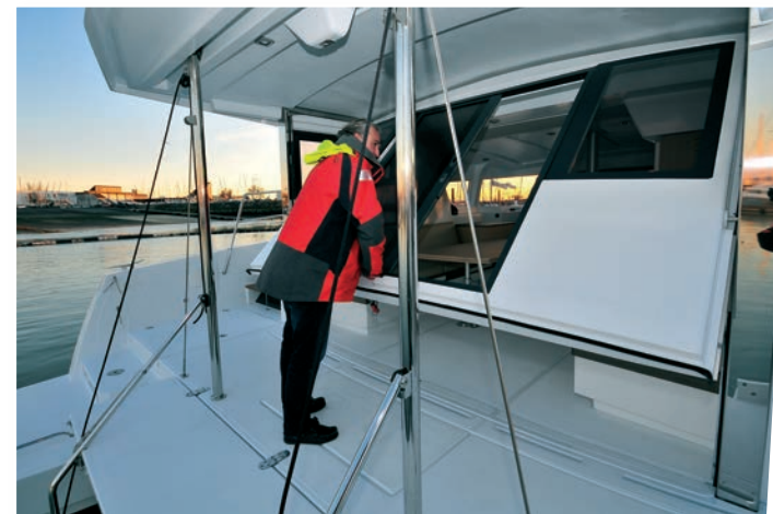
The opening and closing of the aft bulkhead is effortless - the mechanism is assisted by stainless hydraulic rams.
