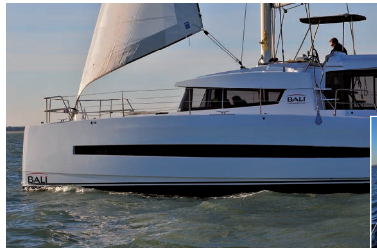
With the rig set further aft, the self-tacking solent is a useful size: the sail turns out to be easy to trim and is powerful. The balance under sail is excellent.
