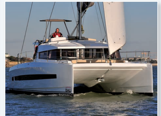
↑ The design and construction of the ski-shape forward is really noteworthy, and the bridgedeck clearance is comparable with the competition. Fine-entry bows, reasonable weight loading, overall intelligent structure and hulls give great results on the water.
