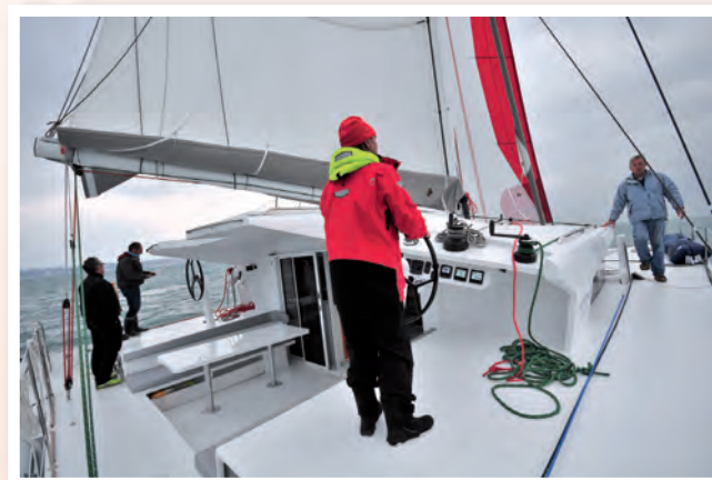
The centered location of the helm stations offers remarkable panoramic visibility and a really sporty position for helming. Note the excellent view of the well-protected electronics
